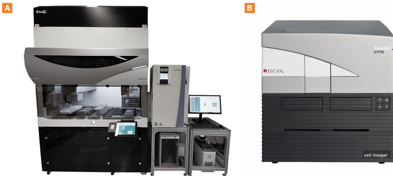
Figure 2. Tecan's Fluent Automation system. The Fluent Automation Workstation (A.) was integrated with the Cytomat 2 C450-LiN Automated Incubator (B.) to automate the PathHunter PD-1 Signaling Bioassay. The measurement of the chemiluminescent signal was performed with a Spark® Cyto 600.
