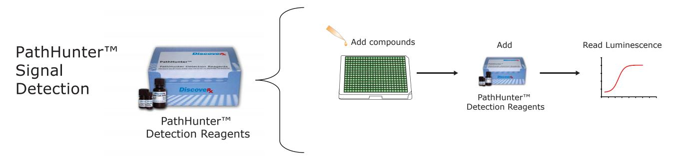
**Figure 2.** The PathHunter Detection Reagents consist of a lysis buffer and substrate mixture that is added as a single solution to stimulated cells. After a short incubation, the PathHunter chemiluminescent signal can be detected using any standard luminometric plate reader.
