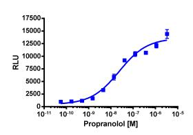
Cell Number/Well:5000Control Compound:PropranololCompound Incubation Time (minutes):OvernightCompound Incubation Temperature (°C):37EC50 for Compound Stimulation (nM):23.7Signal:Background at Agonist Emax:14.9
