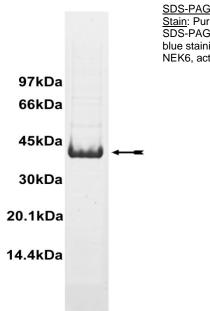
SDS-PAGE and Coomassie Stain: Purity was assessed by SDS-PAGE and Coomassie blue staining using 3µg of NEK6, active.
