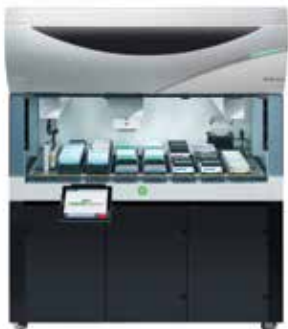
Figure 2. Tecan's Fluent Automation system. A. The Fluent Automation Workstation used to automate the PathHunter CHO-K1 CNR1 bioassay, and B. the Cytomat 2 C450-LiN Automated Incubator that was integrated with the Fluent system.
