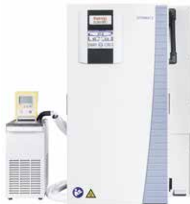
Figure 2. Tecan's Fluent Automation system. A. The Fluent Automation Workstation used to automate the PathHunter CHO-K1 CNR1 bioassay, and B. the Cytomat 2 C450-LiN Automated Incubator that was integrated with the Fluent system.
